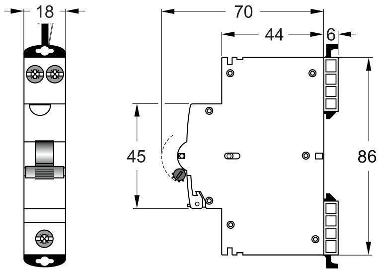
NHP MOD6 Residual Current Device - Short body w/ Overcurrent 6kA 32A 1PN C Curve 30mA Type A Pigtail
